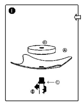
Screw on the retention ring (C) onto the threaded end of tube (B). Insert assembled tube (B) into base (A) and screw on weighted base (D).
