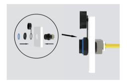
Assemble and tighten in sequence as shown in the figure. Seal with dustcover until ready for use
