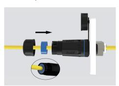
3. Lock the waterproof plug on the cable, then put it into the end of the long tube. Note: The plug is engraved with the word "waterproof" on one side outward.
