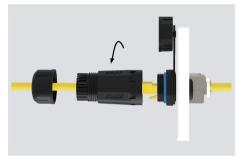
Pass the patch cord through the end cover and the long tube. Then insert the connector. Tighten the long tube.
